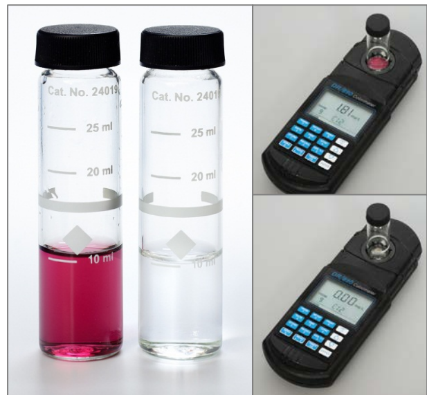
Measuring free available chlorine levels in water using a colorimeter: Pink bottle shows water in which chlorine is detected.
