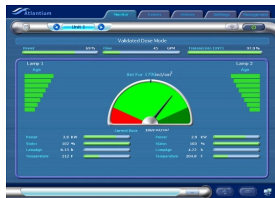
Monitor shows status of critical parameters in real-time, including actual UV dose being delivered.
